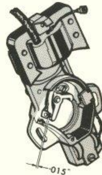
FIGURE 10 Breaker Point Adjustment
